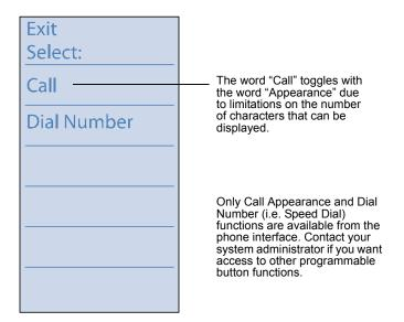
**Step 4** Press the custom key to the left of the function you would like to assign to this key.
